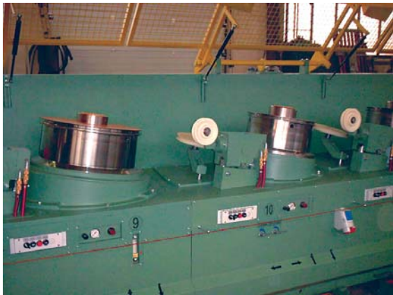
dancer control with individually pivoted guide roll on top of capstan
