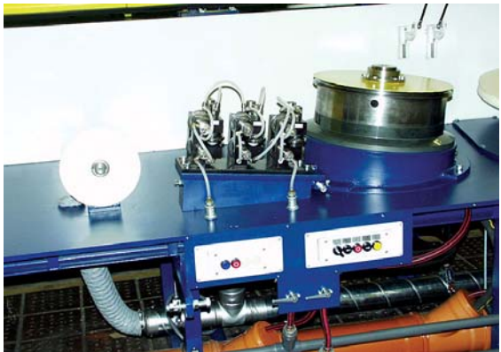
reduction of cross sectional area by cold rolling with compact cassettes
