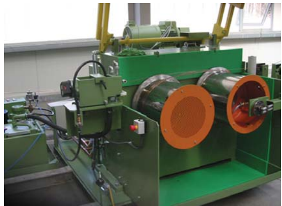
Tandem capstan arrangement for drawing of profile wire and wire with highly sensitive surface like spectacle frame wire
