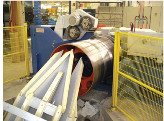
Capstan with disconnectable head for wire guidance on to rotating carrier reel
