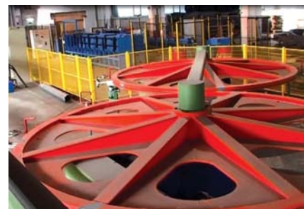
V-grooved capstans ø 4000 mm
