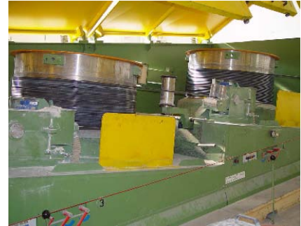
Drawing machine with capstan-ø 1200 mm
