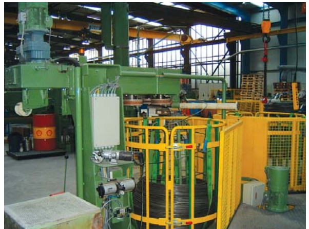
Bending coiler with double take-up on turnstile
