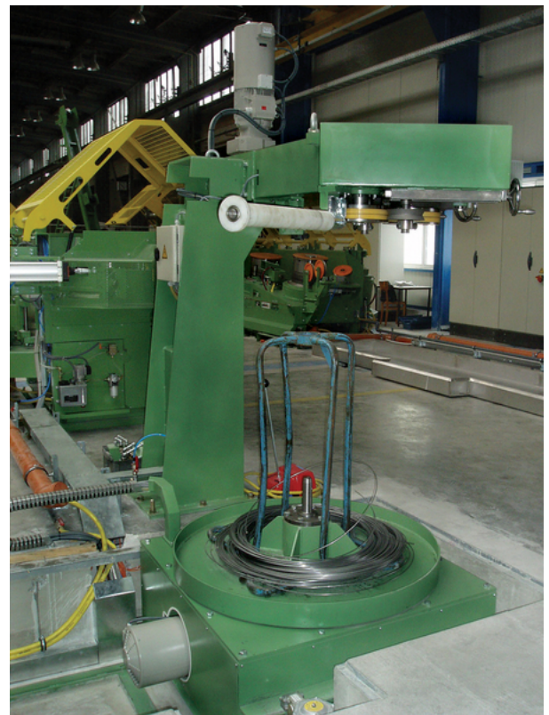
Bending coiler with spiral-type laying system for production of compact coils
