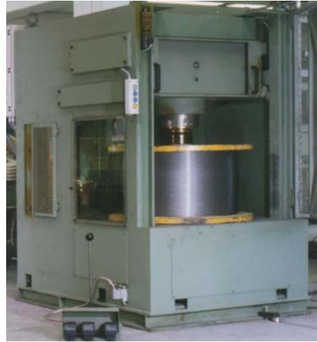
Collapsible spool with incorporated stripping device and adjustable traversing width for "turn by turn" and "Layer on Layer" spooled wire
