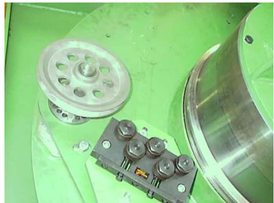
Coiling rotor with straightening device and coiling capstan with casting rim
