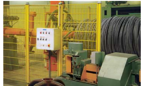
Pay-off with operating panel and wire pointing machine
